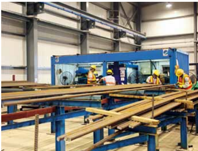
The cut-and-bend factory at our West Kowloon Terminus Station North project is the first in Hong Kong to use computerised scheduling and automated cutting, bending and sorting.
